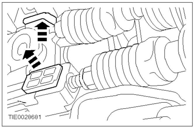
**c** 8. Release the catches for the gearshift cable and selector cable.
