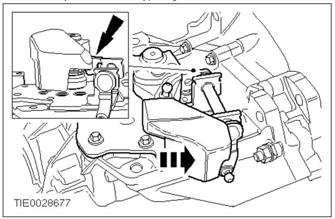
**c** 11. Shift the transmission into neutral (gearshift cables not shown).
