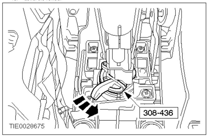
C 14. Turn the special tool counter-clockwise through approx. 45 degrees in order to release the selector mechanism.
