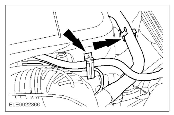
26. Attach the positive crankcase ventilation (PCV) hose and the vacuum hose to the engine cover.
