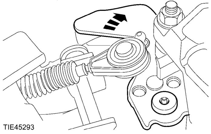
**c** 19. Shift the transmission into 3rd gear.
